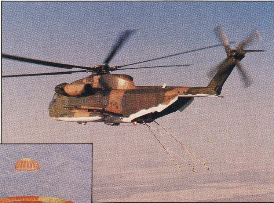
With its poles deployed, a 6514th HH-53C positions itself to snag an air-launched cruise missile (left), which descends beneath a special parachute (far left).
